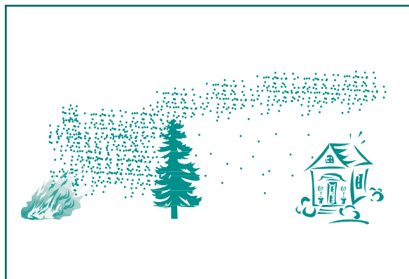
Figure 6.1 Windbreaks act as filters to ember attack
